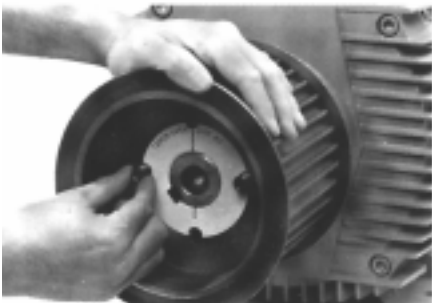
Step 3: tighten screws finger tight
