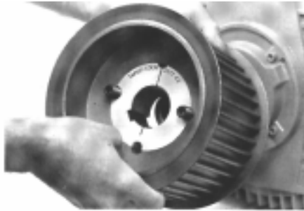
Step 2: insert screws and locate on shaft
