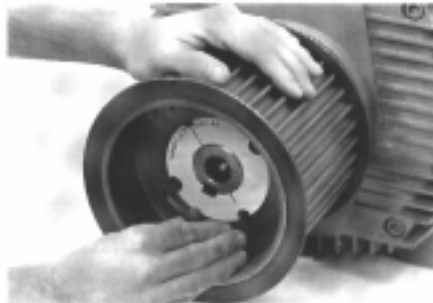
Step 4: tighten screws alternately
