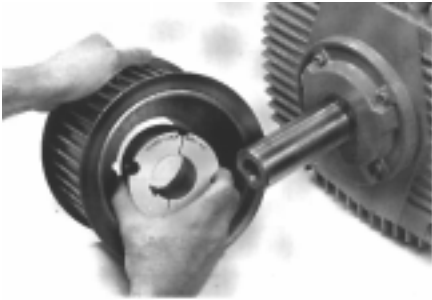
Step 1: insert bush into pulley
